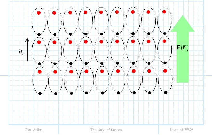
Note since the polarization vector is a **constant**, the equivalent volume charge density is **zero**:
