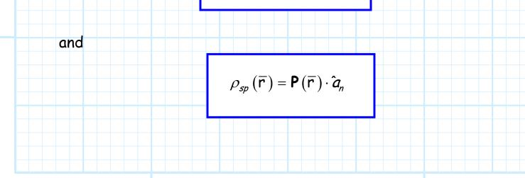
The subscript p (e.g.,  $\rho_{vp}$ ,  $\rho_{sp}$ ) indicates that these functions represent **equivalent charge densities** due to the due to the **dipoles** created in the dielectric.
